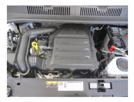
2. Unplug the wiring loom from the map sensor housed in the boost pipe. If your vehicle has an extra breather hose remove this from the boost pipe by pressing in both tabs.
