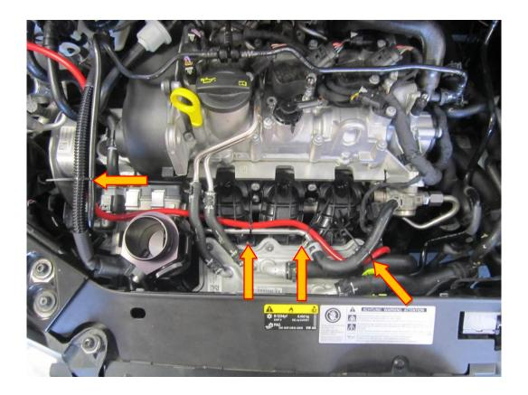
15. Prepare the silicone hose as shown in the picture below. Fit the valve to the hose and secure it with the provided hose clamp using a 7mm socket and rachet or a flat blade screwdriver. Next, loosely place the two larger hose clamps at each end of the hose ready to secure the intake hose to the Forge Motorsport billet couplers.
