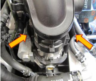
5. Remove the boost pipe fully from situ.
