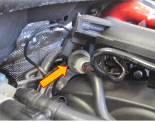
4. Unclip the couplers from the turbo inlet and throttle body while pulling them away from situ.
