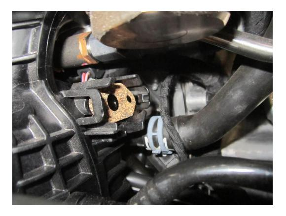
**13**. Fit the boost take off and map sensor into position and fasten with the M5x35 or M6X40 screws provided.
